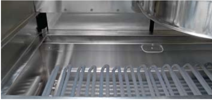
COOLING CHAMBER HEATING ELEMENTS
